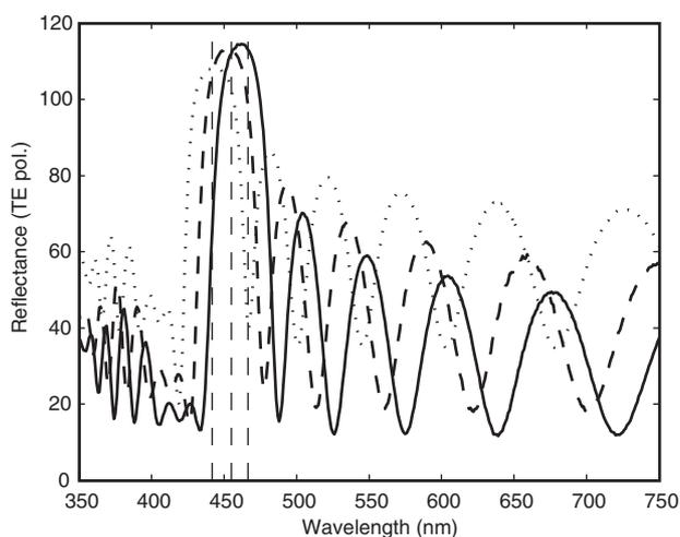
**Figure 3.** Reflectance spectra of WI sample measured at 20° (solid curve), 40° (dashed curve) and 60° (dotted curve) incidence angle. The polarisation state of the incident light was transverse-electric (TE). Vertical dashed lines indicate the positions of the dominant reflected wavelength as predicted by theory.
