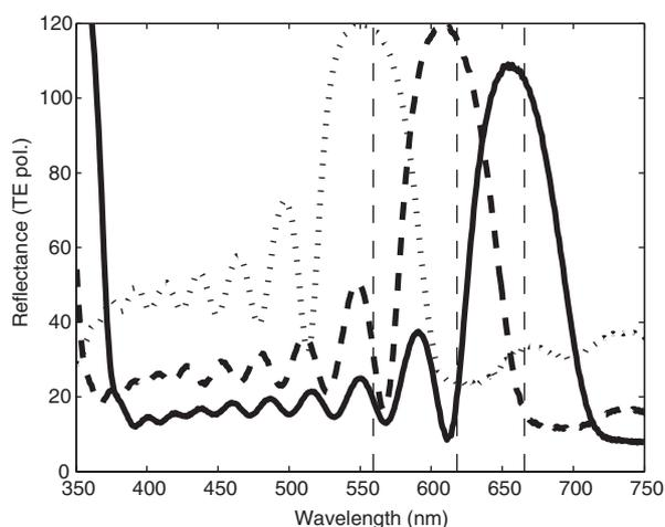
**Figure 2.** Reflectance spectra of SI sample measured at 20° (solid curve), 40° (dashed curve) and 60° (dotted curve) incidence angle. The polarisation state of the incident light was transverse-electric (TE). Vertical dashed lines indicate the positions of the dominant reflected wavelength as predicted by theory.
