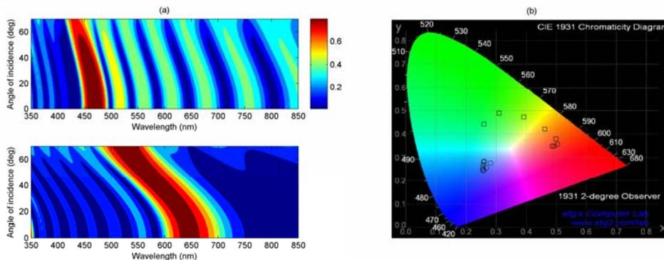
Figure 1. Theoretical reflectance (a) of SiO<sub>2</sub>(n=1.5)/TiO<sub>2</sub>(n=2.7) multilayer films and corresponding chromaticity coordinates (b) as the angle of incidence is increased from 0° to 70°. Hoplia-type design: 14-periods, d<sub>SiO<sub>2</sub></sub>=8 nm, d<sub>TiO<sub>2</sub></sub>=80 nm (a: top, b: circles); Chrysochroa-type design: 8-periods, d<sub>SiO<sub>2</sub></sub>=200 nm, d<sub>TiO<sub>2</sub></sub>=10 nm (a: bottom, b: squares).
